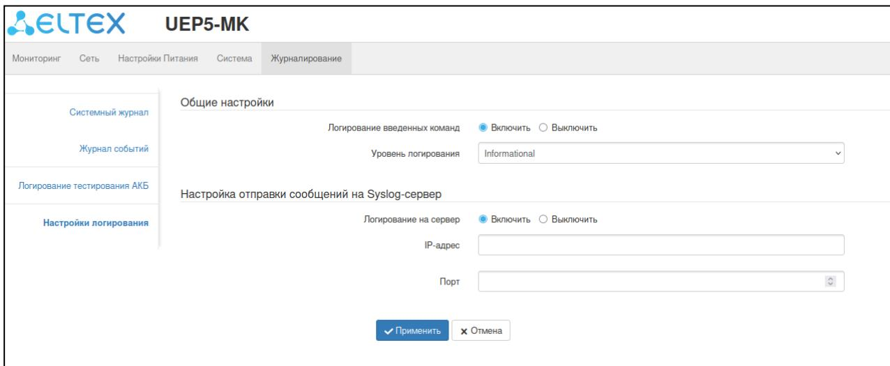
The screenshot shows the UEP5-MK configuration interface with the 'Logging' sub-menu selected. The main menu includes Monitoring, Network, Power Supply Settings, System, and Journaling. The left sidebar lists System Log, Event Log, AKB Testing Log, and Logging Configuration. The right panel displays two sections: General Settings and Syslog Server Message Delivery Configuration.
