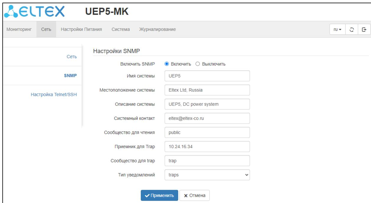
The screenshot shows the configuration interface for the UEP5-MK device. The top navigation bar includes links for Monitoring, Network, Configuration, Power, System, and Logging, along with language and search options. The main menu on the left has sections for Network, SNMP, and Telnet/SSH. The current page is 'Настройки SNMP' (SNMP Settings). The configuration fields include:
